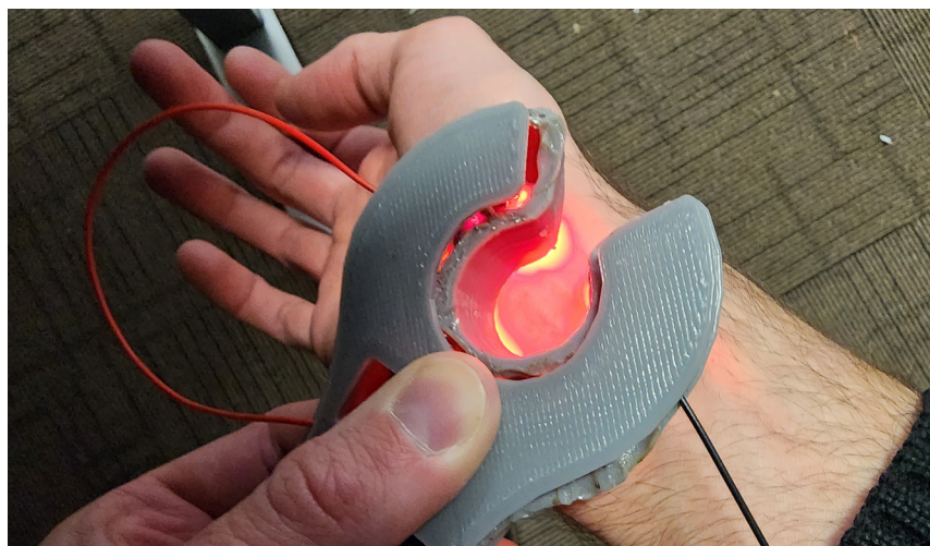
Low-cost 3D-printed medical vein finder prototype photos by Nick Perilli, Innovation Librarian
